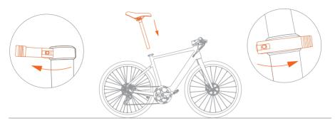
① Open the seat clamp, insert the seatpost.
